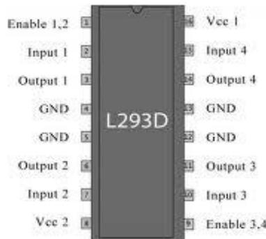
Figure 4: L293D Motor Driver Pin Diagram
