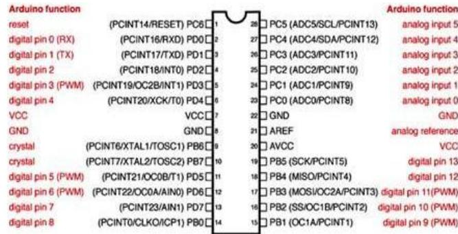
Figure 3: At Mega 8 Pin Diagram
