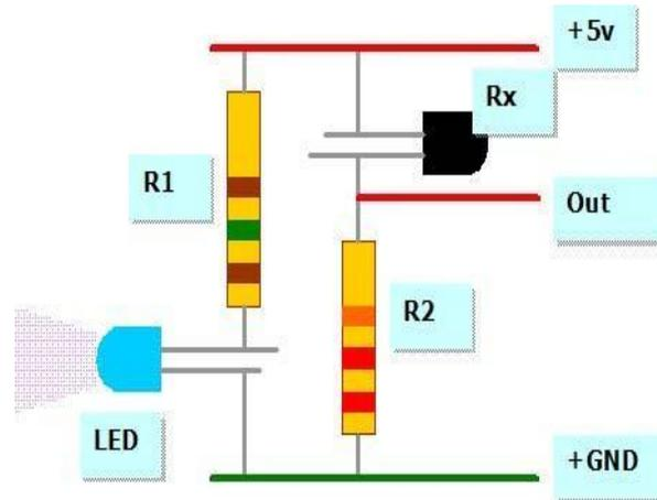
Figure 1: IR Sensor Element
